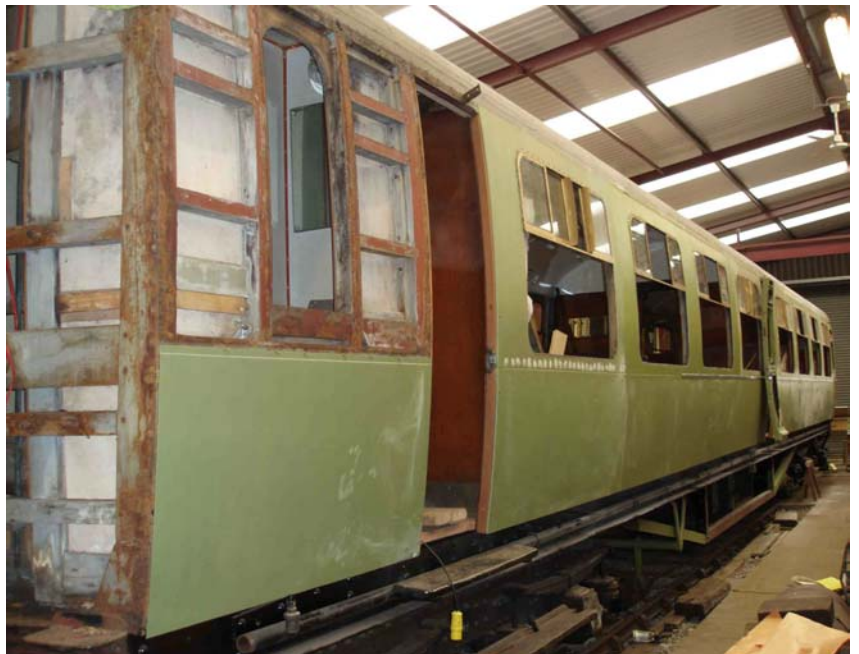
Our Bulleid coach as seen in late March this year. The "missing" upper section of the cladding can be seen top left, with the exposed wooden framing of the Keighley end extreme left. The toplights are glazed, and the waist strip can be seen on the further half of the coach.
