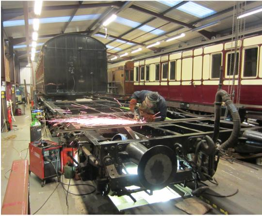
This left one half of the underframe being accessible, with considerations of available space meaning that the other half is still under the (supported) body. This second half will have to take its turn and will involve a trip to Keighley turntable! Closer inspection of the nowaccessible steelwork confirmed that the corrosion problems were indeed limited to the outer edges.
