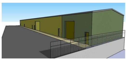
Perspective drawing by our Architect, Steve Brown, showing the intended extension. This is the dark green section to the right, including a second roller shutter door and a further pedestrian access door. This is looking Southwards (that is, towards Oxenhope). The grey area to the left is taken up by the Railway's two sidings (with the Keighley High Level Sewer running underneath them), with the Railway's main line to the left of this.
