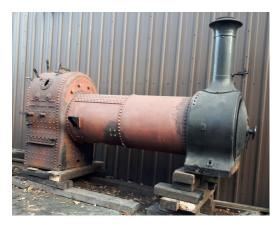
My accompanying photograph shows the boiler standing in Moor Road Yard. It should be noted that, although a modern boiler (built in 2005) it has been riveted, rather than welded as would be normal practice these days. This was done to preserve the historic nature of the locomotive – this boiler is in fact more or less what Manning, Wardle would have had to build in later years. It can be compared with the original boiler (also at Moor Road) to see the engineering advances.
