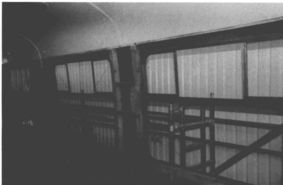
Purchased with much-appreciated Grant assistance from the Yorkshire & Humberside Museums Council, our new access staging is just visible through the windows of the Bulleid coach. Note the just-fitted sliding window toplight frames. Photo: John Wallis
