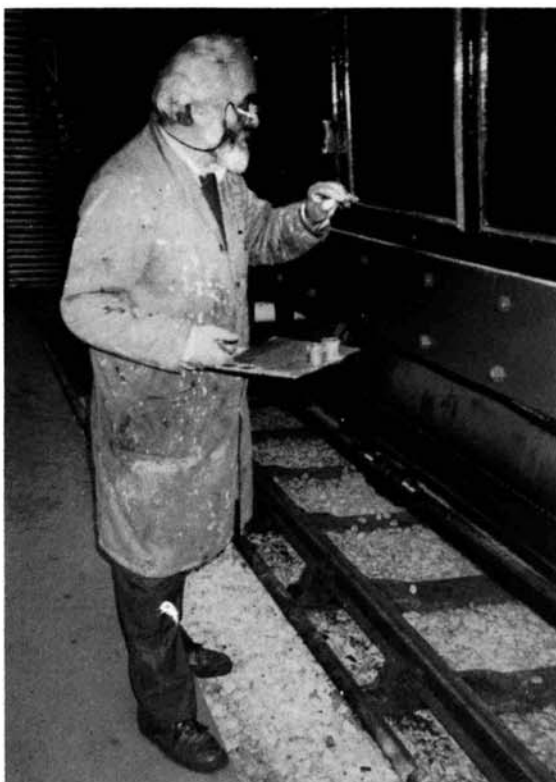
Bob Timmins at work – here, lining-out the lower part of one of 2856's doors
