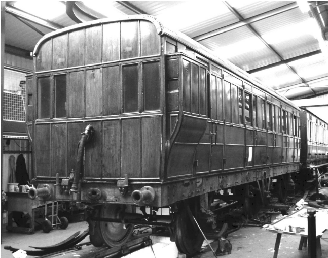
Left: the Great Northern six-wheeler; less buffers, drawgear, stepboards, stepboard brackets: work very much "in progress". Right: underneath this coach – handbrake linkage (complete with new pivot pins) is to the top right; elsewhere cleaning, painting and other general maintenance work is well in hand.
