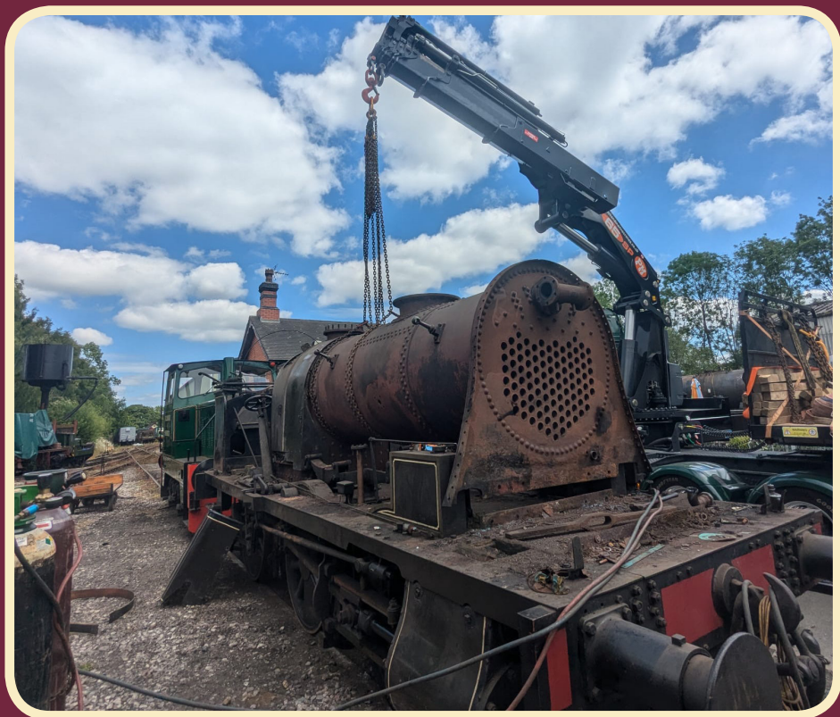
Bellerophon Boiler going to Cromford. Photo: John Eastwood
